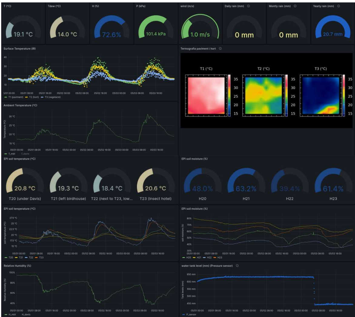
Figure 1. Snapshot of a Grafana dashboard from one of the studied green roofs. From top to bottom, the first row shows real-time gauges for weather data, including daily, monthly and yearly rainfall. The second row shows, on the top-left side, a 72 h time series for surface temperature of three different systems, conventional ceramic roof tiles (green), dry substrate without vegetation (yellow) and a vegetation-covered parterre (blue); and on the bottom-left side the ambient temperature. The right side of the second row shows real-time (8x8 px) thermographic images of the three aforementioned surfaces, in the same order from left to right. The third row shows real-time gauges for soil temperature (left) and moisture (right) at four different locations, all of them buried in periodically irrigated substrate. The fourth row shows time series for all these eight gauges. The fifth row shows time series for the ambient humidity (left) and for the water tank levels where rainfall is harvested (right). This is only a part of the dashboard, where other gauges and time series have been omitted for the sake of simplicity.
